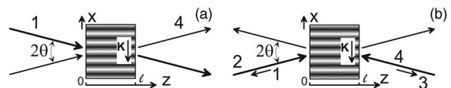
Fig. 1. Scheme of (a) beam coupling and (b) DPCM geometries. In (a) signal beam 4 is amplified at the expense of coherent pump beam 1. In (b) the path difference of beams 4 and 2, which impinge upon the sample, is larger than the laser coherence length, and new beams 3 and 1 are generated. The structure of the index grating is shown inside the samples.
