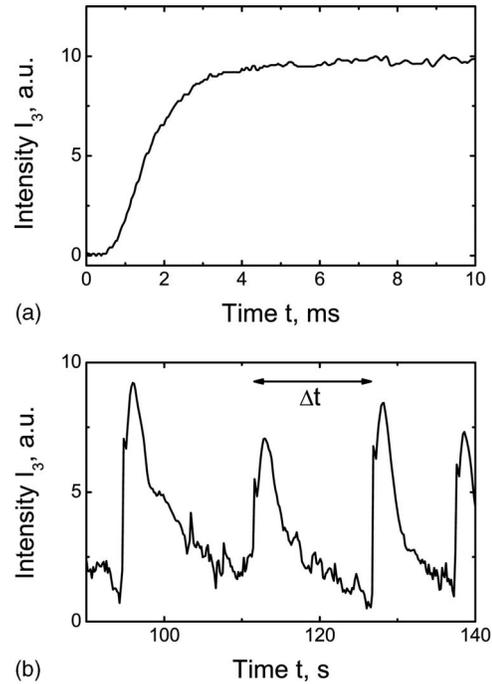
Fig. 3. Temporal dynamics of the oscillation intensity (a) just after exposure of a virgin sample and (b) for well-established oscillation ( $\Lambda = 1.4$   $\mu$ m,  $r = 4$ ). Note the difference in the time scale for the two frames.
