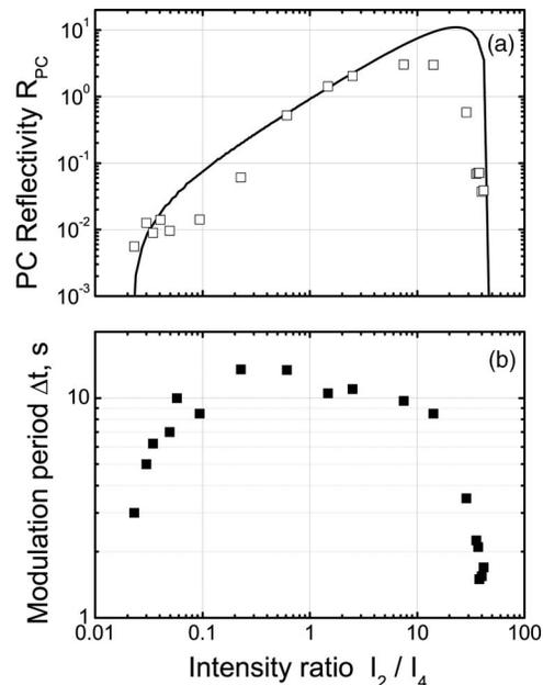
Fig. 4. (a) Phase-conjugate reflectivity and (b) period of intensity variation versus beam ratio for  $\Lambda = 1.4$   $\mu$ m. The solid line is the dependence calculated in plane-wave approximation [2] for lossless medium and  $\Gamma \ell = 8$ .
