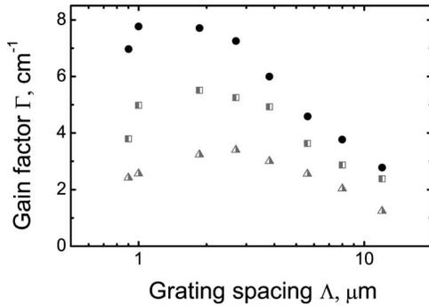
Fig. 2. Grating-spacing dependence of the gain factor  $\Gamma$  at 647 nm for intensities of the pump wave 0.1, 1.0, and 10 W/cm<sup>2</sup> (triangles, squares, and dots, respectively.)
