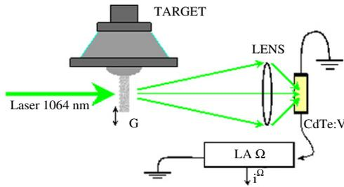
**Figure 2.** Schematic representation of the setup. The target is a diffusing glass plate **G** attached to the cone of a commercial loudspeaker; the photocurrent is collected by lateral electrodes on the photorefractive crystal and fed to a lock-in amplifier tuned to  $\Omega$ . (This figure is in colour only in the electronic version)
