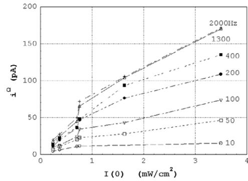
**Figure 7.** First harmonic photocurrent component  $i^\Omega$  as a function of the irradiance for different frequencies, always for  $\delta = 0.3$ .
