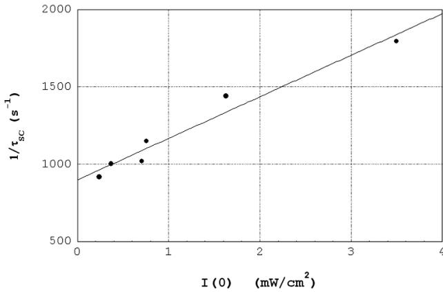
**Figure 6.** Inverse response time as a function of the irradiance at a fixed  $\delta = 0.3$ .
