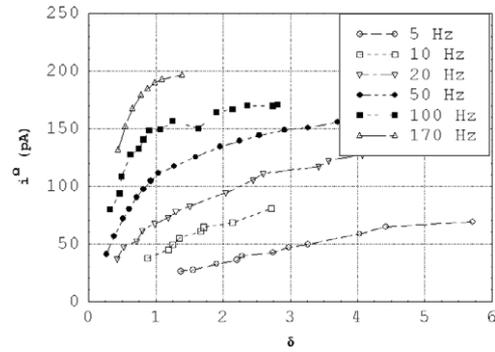
**Figure 4.** First harmonic photocurrent component  $i^\Omega$  as a function of the normalized vibration amplitude  $\delta$  for different frequencies in the range 5 Hz–170 Hz and a fixed irradiance  $I(0) = 3.78 \text{ mW cm}^{-2}$ .
