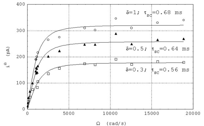
**Figure 5.** First harmonic photocurrent component  $i^\Omega$  data as a function of frequency for  $\delta = 1, 0.5$  and  $0.3$ , with  $I(0) = 3.78 \text{ mW cm}^{-2}$ . The continuous lines are the best fitting with equation (3), leading to the corresponding different values for  $\tau_{SC}$  indicated in the figure.
