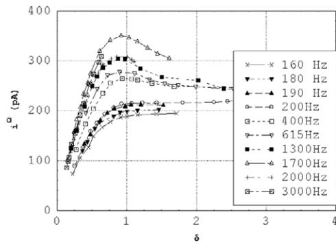
**Figure 3.** First harmonic photocurrent component  $i^\Omega$  as a function of the normalized vibration amplitude  $\delta$  for different frequencies in the range 160 Hz–3000 Hz and a fixed irradiance  $I(0) = 3.78 \text{ mW cm}^{-2}$ .
