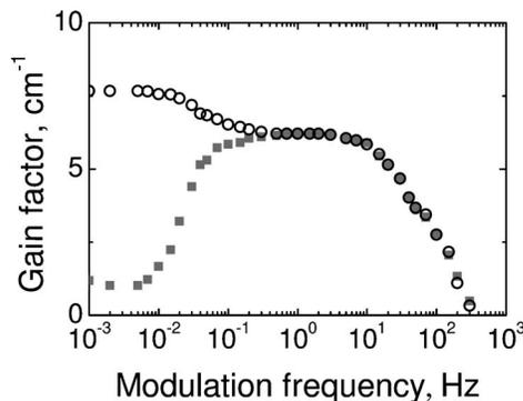
Fig. 2. Modulation frequency dependence of the transient gain factor (open circles) for periodic  $0-\pi-0-\pi-0-\pi-$  phase modulation and the steady-state gain factor (gray squares) for sawtooth phase modulation.
