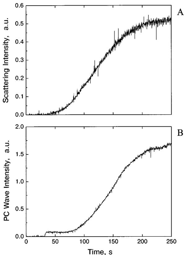
Fig. 4. Temporal development of A, the total intensity of the conical scattering, and of B, the phase-conjugate (PC) beam intensity. Two extraordinary pump waves permanently illuminate the sample while the signal wave is switched on at  $t = 30$  s.
