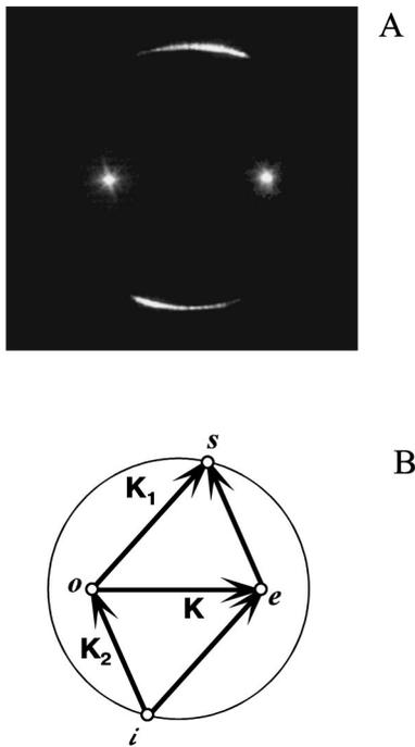
Fig. 2. A, Intensity distribution on the screen placed 20 cm behind the sample in the direction of the propagation of waves 1 and 3. Two bright dots mark the positions of the transmitted incident waves. B, Grating vector diagram to explain the parametric conical scattering. The tips of the wave vectors of the signal (3) and the pump (1) waves are labeled *o* and *e*; the tips of the wave vectors of the scattered waves are labeled *s* and *i*.
