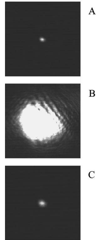
Fig. 3. Far-field intensity distributions, A, for two pump waves and an initial signal wave; B, for a distorted signal wave; C, for a conjugate beam passing back through the distorter (lens). The divergence of the beam in B is  $\sim 0.5^\circ$ .
