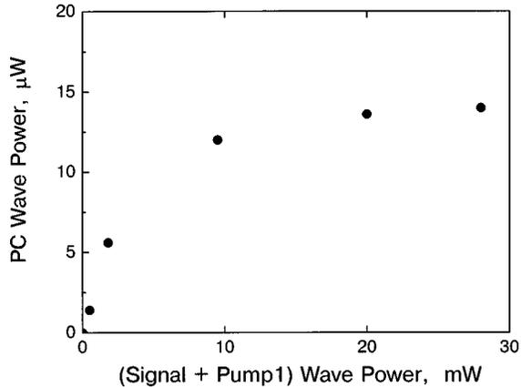
Fig. 5. Steady-state intensity of the phase-conjugate (PC) wave as a function of the overall intensity of copropagating waves 1 and 3. The power of the readout wave 2 is 0.5 mW.
