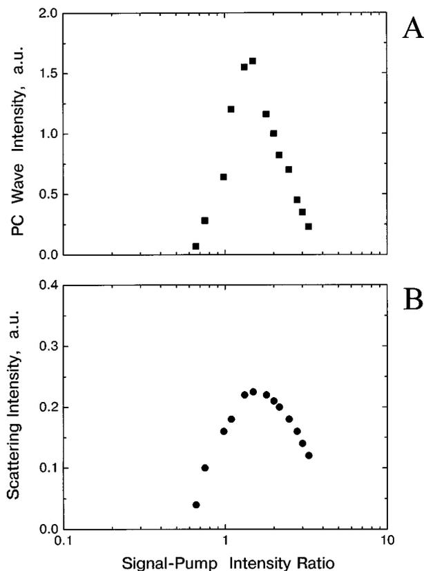
Fig. 6. A, Phase conjugate (PC) wave intensity and B, scattered light intensity versus the intensity ratio of the signal wave to the copropagating pump wave. The intensity of the counterpropagating pump wave is 10 times smaller than that of the copropagating pump wave.
