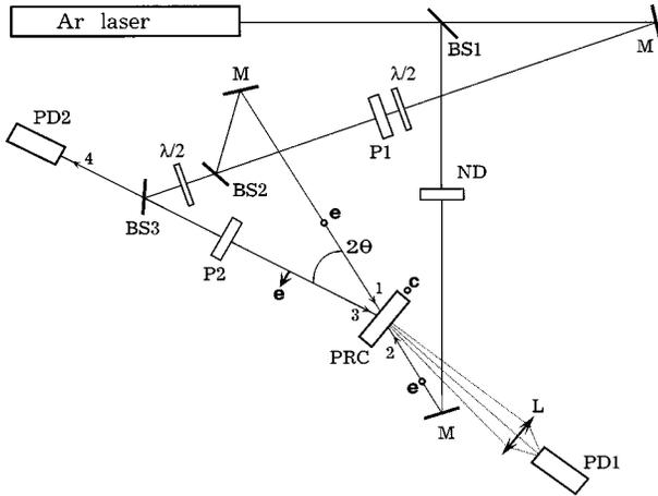
Fig. 1. Schematic representation of the experimental setup: M's, mirrors; PRC, photorefractive crystal; other abbreviations are defined in text.
