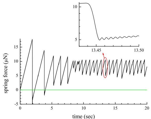
Fig. 2: (Colour on-line) Calculated slider spring force in the stick-slip regime. Parameters as given in the text, and  $g = 0$ . The inset shows the detail of a slip, with the sudden force drop and mechanical ringing oscillations.
