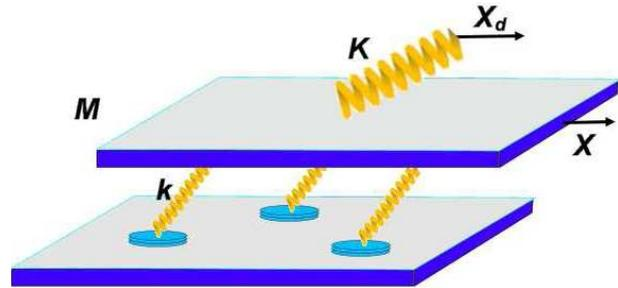
Fig. 1: (Colour on-line) The earthquake-like model.
