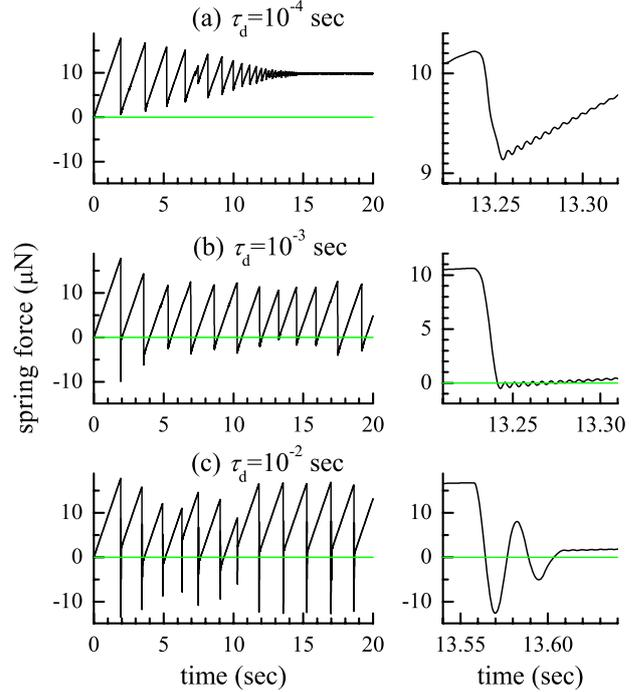
Fig. 4: (Colour on-line) Frictional force  $F(t)$  for different values of the delay time  $\tau_d$ . Despite the soft spring constant  $K = 97 \text{ N/m} \ll K^* \sim 10^5 \text{ N/m}$ , stick-slip is only found for sufficiently large  $\tau_d$ .
