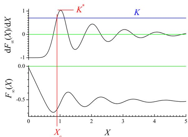
Fig. 3: (Colour on-line) Force vs. displacement of the rigidly coupled slider ( $K = \infty$ ) with  $\Delta f_s/f_s = 0.2$  and  $Nk = 1$ . The oscillations are due to the alternate prevailing of contact breaking ( $|F_\infty|$  drops) and contact reforming (rises). Their damping leads finally to smooth sliding.
