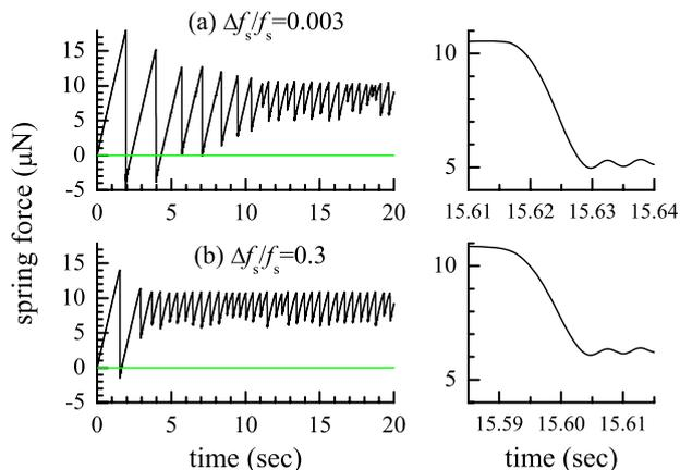
Fig. 5: (Colour on-line) Dependence  $F(t)$  for different values of the dispersions  $\Delta f_s$ .
