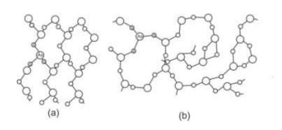
The structures of  $As_2S_3(a)$  – crystalline phase, (b) – glassy phase.
