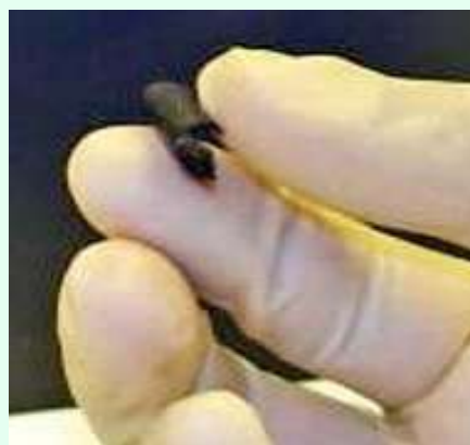
Fig. 7. Thin and flexible paper battery of cellulose-based implanted nanotubes as electrodes
