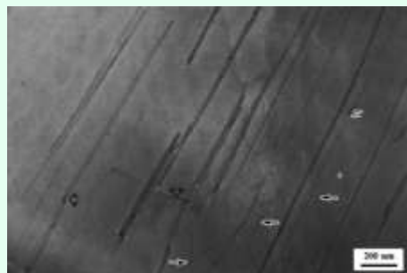
Fig. 4. Alignment of nanotubes in polymer matrix following cutting with microtome: arrows indicate buckled nanotubes
