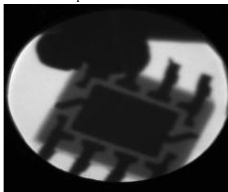
Fig. 1. X-ray image of microchip
