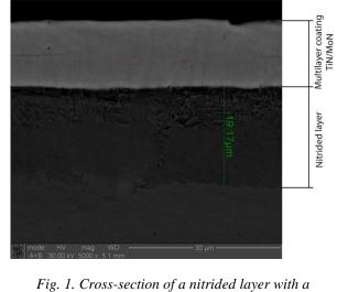
Fig. 1. Cross-section of a nitrided layer with a multilayered TiN/MoN coating
