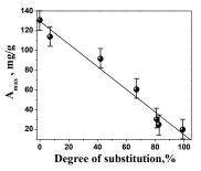
It's been shown that free silanol groups play a principal role in adsorption of polyvinypyrrolidone onto nanosilica surface. The value of the maximal adsorption (monolayer capacity) on hydrophobic silica, where the surface silanol groups are completely replaced by trimethylsilyl ones, has been found to be approximately 6.5 times smaller than that in the case of the parent hydroxylated sample.
