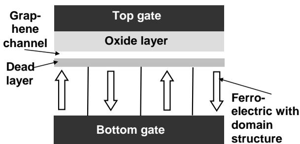
**Figure 1.** Schematics of the nano-structure "graphene channel - ferroelectric substrate with domain walls"
