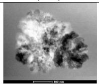
Fig. 1. Microstructure cut-section view of Ga<sub>2</sub>As<sub>28</sub>Se<sub>50</sub>Te<sub>20</sub> glass
