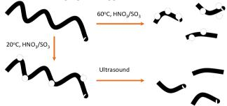
The US-NTs prepared at 60 °C are strongly hydrophilic, but no excitonic peaks were seen in absorbance and PL spectra. The US-NTs done at 20°C are more hydrophobic and the excitonic peaks are clearly seen. These differences are caused by high concentration of lateral defects in the NTs after oxidation at 60°C, while the defects formed at 20°C mainly serve as the break-points for NTs cutting by the ultra sound.
