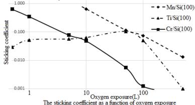
It is clearly seen that the initial oxidation rate for the silicon surface with transitional metal submonolayer decrease from Mn and Cr to Ti.
