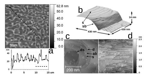
In this contribution we employ a scanning tunneling microscopy in ultra-high vacuum to study the transformation from an atomically flat Ru(0001) to heterogeneous Ru- $RuO_2$  nanostructured surface and investigate its morphological changes as a result of interaction with  $O_2$ , CO and  $Cl_2$ .
