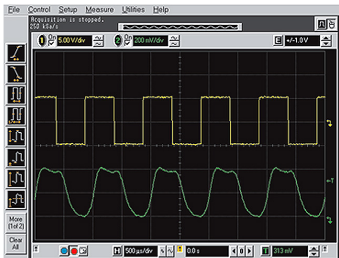
FIGURE 4 — Optical response of FLC cell on the rectangular driving signal with an amplitude 5 V and period of 1 msec.
