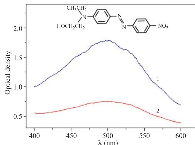
Fig. 2. Polarization spectra of sandwich type LC cell ( $d = 15 \mu\text{m}$ ) for parallel alignment filled with LC E7 doped with the dye DR1 (0.5 wt.%). Spectra 1 and 2 correspond to the light polarization direction parallel and perpendicular to the direction of LC alignment. Since LC E7 does not absorb light in the selected spectral range, the measured spectra reflect absorption of the dichroic dye DR1. Inset shows chemical structure of the dye.
