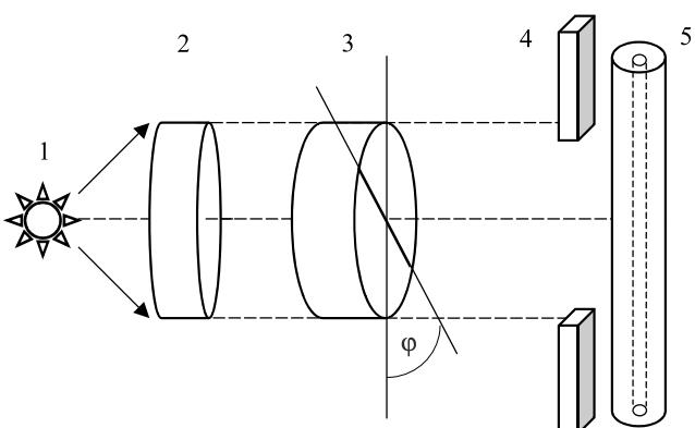
Fig. 1. UV irradiation setup: UV lamp (1), collecting quartz lens (2), UV polarizer (3), mask (4), capillary (5).
