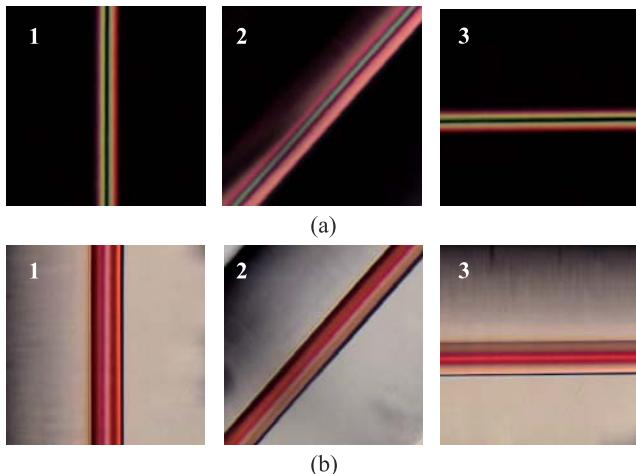
Fig. 8. Microphotographs of the capillary sample filled with the dyed LC E7 forming escaped radial alignment configuration [Fig. 5(d)]: (a) observation between two of crossed polarizers with, accordingly, vertical and horizontal polarization axis:  $\alpha = 0^\circ$  (1),  $\alpha = 45^\circ$  (2),  $\alpha = 90^\circ$  (3); and (b) observation in vertically polarized light:  $\alpha = 0^\circ$  (1),  $\alpha = 45^\circ$  (2),  $\alpha = 90^\circ$  (3).
