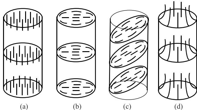
Fig. 5. LC alignment configurations realized in cylindrical microcapillaries with (a–c) planar and (d) homeotropic anchoring conditions: (a) axial configuration, (b) transversal configuration, (c) tilted configuration, (d) escaped radial configuration.
