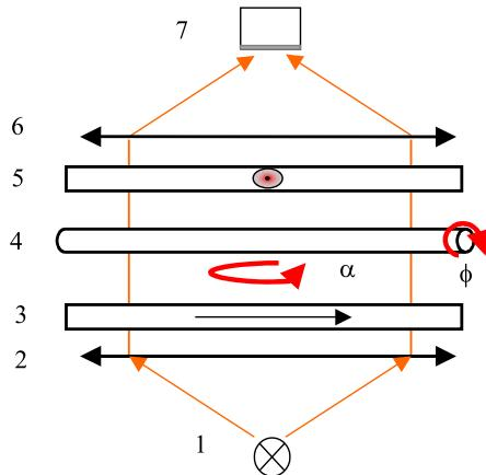
Fig. 3. Scheme demonstrating sample rotation directions during inspection in polarizing microscope: light source (1), condenser (2), polarizer (3), sample (4), analyzer (5), objective (6), camera (7).
