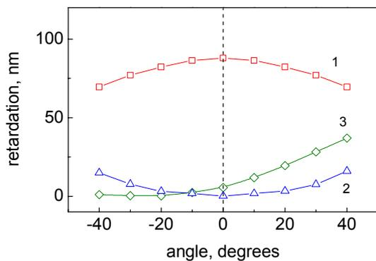
**Fig. 4. Retardation vs rotation angle obtained for (1) p-RM, (2) h-RM, and (3) t-RM.**
