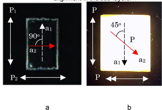
**Fig. 6 Photographs of two-layer RM films with planar alignment. Alignment axes in the layers form angle (a)  $90^\circ$  and (b)  $45^\circ$ .**
