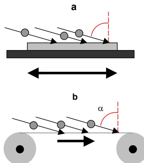
Fig. 2 Particle beam processing scheme for (a) rigid substrates and (b) flexible strips.
