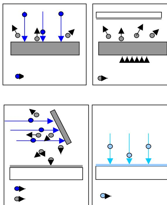
**Fig. 1. Particle beam etching and deposition processes:**
