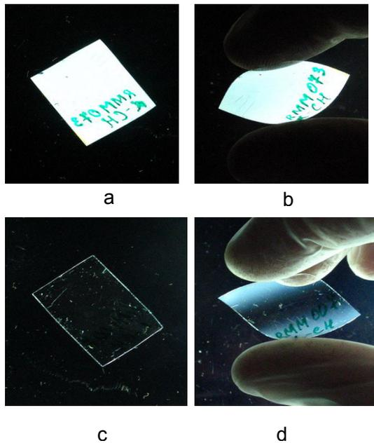
**Fig. 3. Photographs of RM films with (a, b) planar and (c,d) homeotropic alignment deposited on isotropic plastic (TAC) substrates. The films have optical properties of +A and +C films, respectively.**
