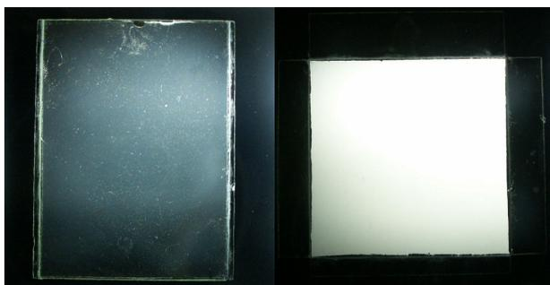
Fig. 5. Photos of 12x15 cm symmetric cells ( $d = 20 \text{ mm}$ ) based on plasma treated PI substrates viewed between crossed polarizers. The cells are filled with LC ZLI2293. a – twist angle is zero; b – twist angle is 90. Irradiation conditions:  $a = 700$ ,  $j = 8 \text{ mA}/\text{cm}^2$ ,  $E = 600 \text{ V}$ .
