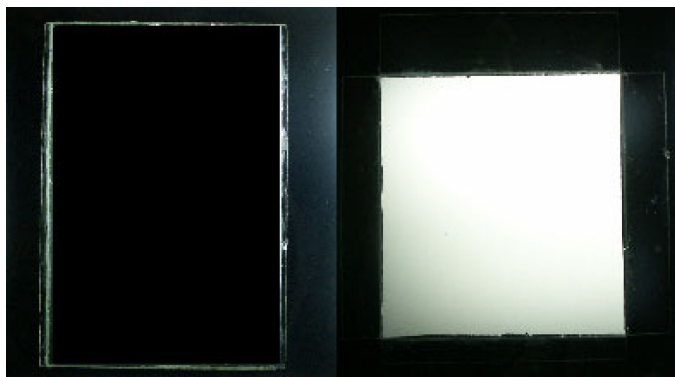
FIGURE 7 — Photos of 120 \times 150 \text{ mm}^2 symmetric cells ( d = 15 \text{ }\mu\text{m} ) based on plasma treated PI substrates viewed between two crossed polarizers. The cells are filled with LC ZLI2293. (a) Twist angle is zero; (b) twist angle is 90^\circ . Irradiation conditions: \alpha = 70^\circ , j = 8 \text{ }\mu\text{A}/\text{cm}^2 , E = 600 \text{ V} , 2 min (a) and 10 min (b).
