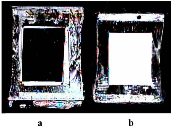
Figure 3. Photos of two combined cells filled with LC 5CB having rubbed PI substrate as a reference substrate and plasma treated glass slide as an object substrate. The object substrates are irradiated through the mask opening rectangular area in the middle of the substrate. The cells are placed between pair of crossed polarizers. The photos exhibit LC alignment in mode 1 (a) and mode 2 (b).
