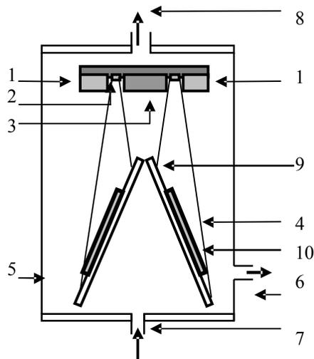
Figure 1. Scheme of anode layer thruster and irradiation method. 1-outer cathode and N pole; 2 - anode; 3 - inner cathode and S pole; 4 - plasma flux; 5 - body of vacuum chamber; 6-8 - gas valves; 9 - substrate holder; 10 - substrate.
