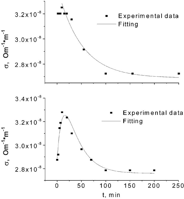
**FIGURE 3** Experimental and fitting curve  $\sigma(t)$  corresponding to the cell irradiated and filled in air. a) non-irradiated cell; b) cell irradiated 20 min.
