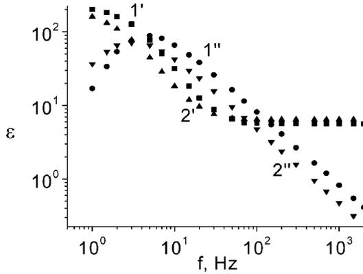
**FIGURE 2** The frequency dependencies of real  $\epsilon'$  (1', 1'') and imaginary  $\epsilon''$  (2', 2'') parts of dielectric permittivity for two regimes of cell filling. In regime 1 (curves 1' and 1'') the cell is irradiated and filled with LC in air. In regime 2 (curves 2' and 2'') the cell was irradiated and filled with LC in vacuum  $10^{-2}$  Torr. The cell gap is  $13.5\ \mu\text{m}$ .
