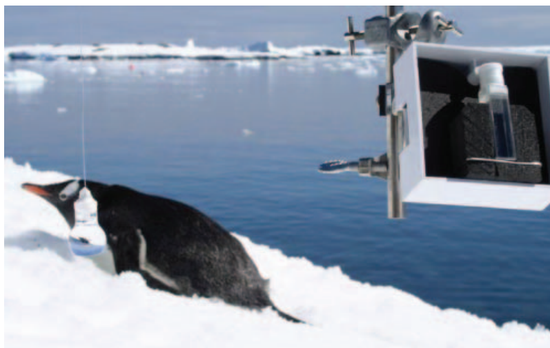
Figure 2. Exposure of provitamin D 3 solution in spherical and quartz cuvettes at the Vernadsky station in Antarctica.
