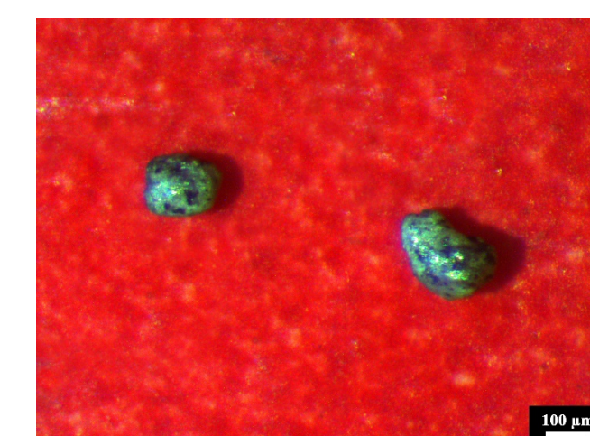
Fig. 3. Polyethylene covered with CNTNiFe
