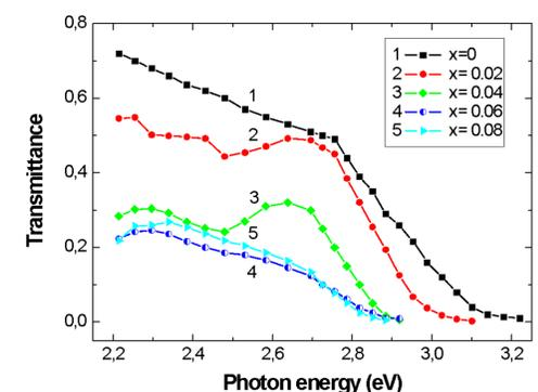
Fig.8 Transmittance spectra of  $Zn_{1-x}Co_xO$  thin films on different substrates at room temperature
