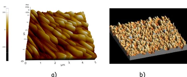
Fig.2. 3D AFM images of the  $Zn_{1-x}Co_xO$  (a) and  $Zn_{1-x}Ni_xO$  (b) thin films
