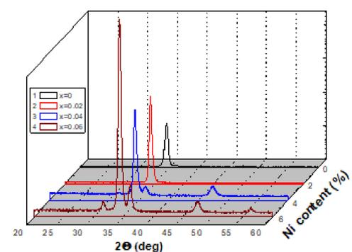
Fig. 7. X-ray diffraction spectra of Ni doped ZnO thin films with various doping level
