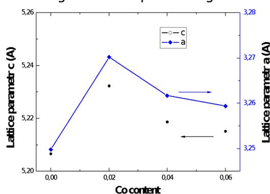
Fig. 5. Dependence of lattice parameter on Co content in  $Zn_{1-x}Co_xO$  thin films
