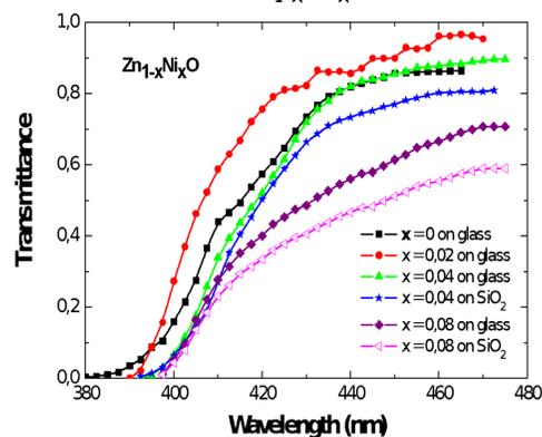
Fig. 6. Transmittance spectra of  $Zn_{1-x}Ni_xO$  thin films on different substrates at room temperature
