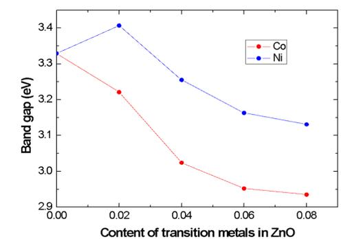
Fig. 9. The energy band gap of  $Zn_{1-x}Me_xO$  thin films as a function of Co and Ni- content.
