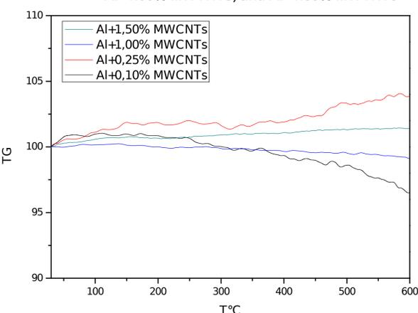
We notice that all for samples present a good stability over the whole temperature range, however, there's some mass change for the samples containing low concentrations of MWCNTs. For the sample Al + 1.5% MWCNTs, the curve shows that the mass remains practically constant over the whole temperature range. We conclude that the introduction of MWCNTs improves the mass stability of the nanocomposites.
