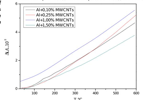
Coefficient of thermal expansion of Al+0.10% MWCNTs, Al+0.25% MWCNTs, Al+1.00% MWCNTs, and Al+1.50% MWCNTs
