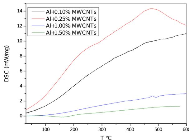
The two highest concentrations led to calorimetric curves having the same shapes. Those of 0.1% and 0.25% MWCNTs gave intense DSC curves. the comparative study between the DSC of the 4 samples shows that the 1.5% MWCNTs nanocomposite has the lowest DSC compared to that of 0.25% which has the highest heat capacity.
