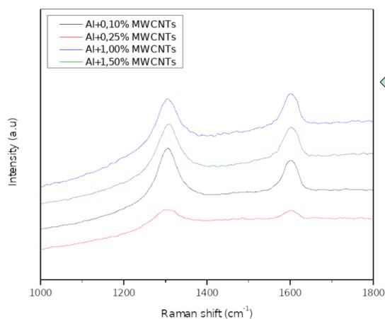
We notice that the ratios ID/IG have increased with the increase in MWCNTs concentration. This means that the quantity of defects has also increased with increasing concentration. This can lead to a destruction of the MWCNTs. on the other hand; the ID/IG values remain included in the domain (0.5, 3) of the literature..
