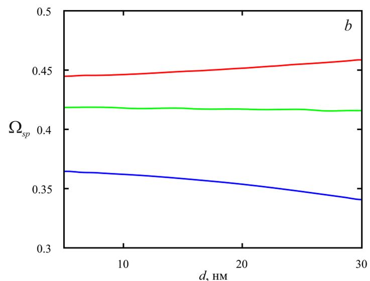
Fig. 2. Dependencies of SPR frequencies for structures  $\text{SiO}_2@\text{Au}$  (a) and  $\text{SiO}_2@\text{Ag}$  (b) at  $a = 10$  nm and  $b = 40$  nm on the distance between the cylinder axes
