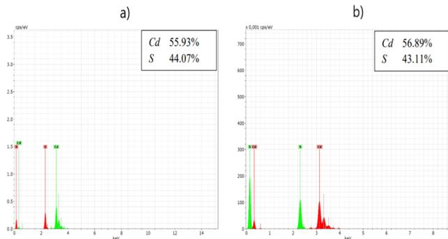
**Fig. 1. The EDS spectrum of CdS/glass thin films: a) sample 1b, b) sample 2b.**
