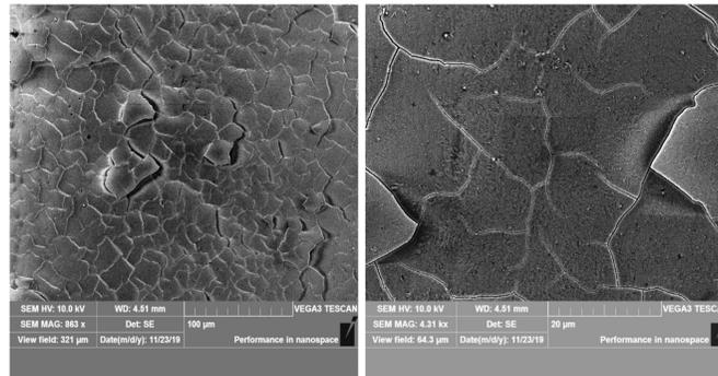
**Fig. 2. CdS sample 1b ( $T_s = 470$  K,  $T_E = 880$  K,  $\tau = 90$  sec,  $d = 560$   $\mu$ m).**
