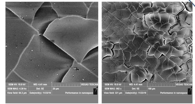
**Fig. 3. CdS sample 2b. ( $T_s = 470$  K,  $T_E = 880$  K,  $\tau = 60$  sec,  $d = 420$   $\mu$ m).**
