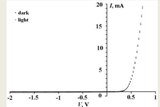
Fig. 5. Light  $I$ - $V$ -characteristics of the heterojunction  $p$ -CuCoO<sub>2</sub>/ $n$ -Si at  $T=295$  K.
