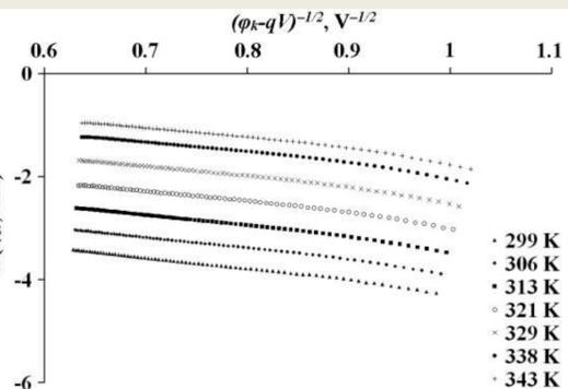
Fig. 4. Temperature dependences of reverse  $I$ - $V$ -characteristics for  $p$ -CuCoO<sub>2</sub>/ $n$ -Si heterostructure.
