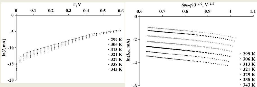
Fig. 3. Dependences  $\ln I = f(V)$  at forward biases applied to the  $p$ -CuCoO<sub>2</sub>/ $n$ -Si heterostructure at different temperatures.
