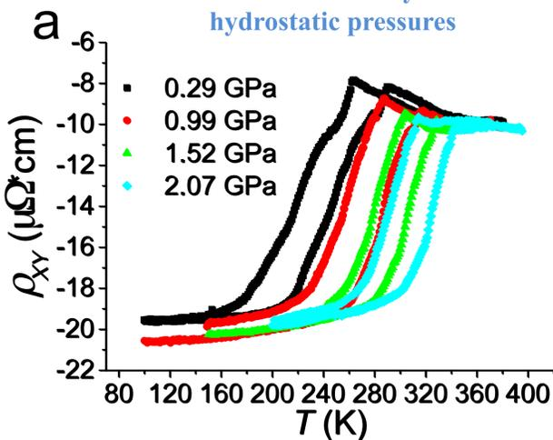
Figure 2. Temperature dependences of longitudinal resistivity in Ni<sub>45.4</sub>Mn<sub>40</sub>In<sub>14.6</sub> at different hydrostatic pressures. The inset shows the variation of the martensite start temperature with pressure.
