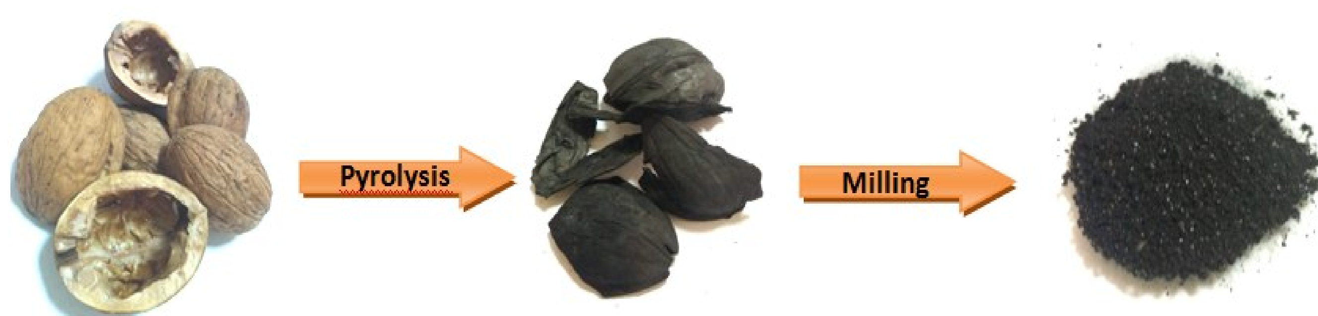
Fig. 1. Schematic illustration of the synthesis of NPC from walnut shell
