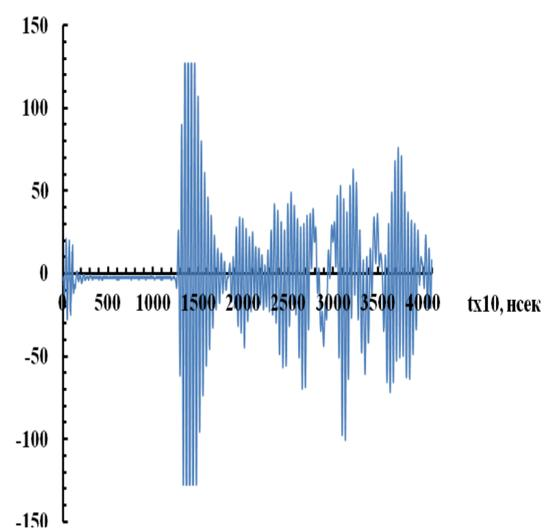
Fig. 6. Oscillogram of impulses with quasi-longitudinal polarization  $V_{\parallel[001]}$  in  $\text{SiO}_2$
