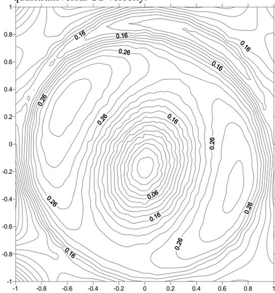
Fig. 4. Stereoprojection of isolines of Poisson coefficient  $\mu$   $\text{SiO}_2$
