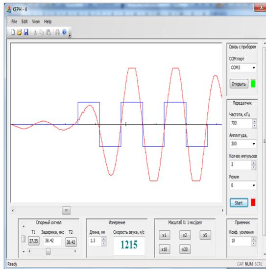
Fig. 3. Illustration of the window for processing data of quasi-transversal elastic wave velocity measuring  $V_{\perp} = 1215$  m/sec in nanocomposite polyamide-6 (PA-6)  $(\text{NH}(\text{CH}_2)_5\text{CO})_n$  + 1.7% methylene dye blue squaring
