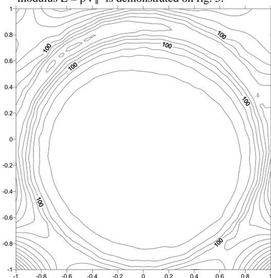
Fig. 5. Stereoprojection of isolines of the elastic modulus  $E$   $\text{SiO}_2$
