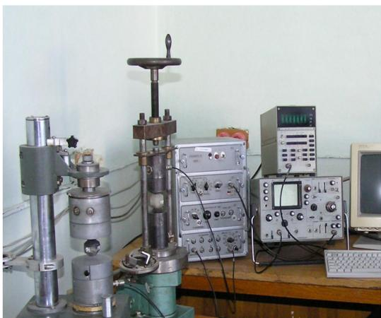
Fig. 2. Ultrasonic equipment KERN-SG for measuring of elastic waves velocities  $V_{\parallel}$ ,  $V_{\perp}$
