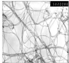
Fig. 1. Group of multiwall carbon nanotubes.
