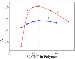
Fig. 2. IR absorption by  $sp^3$  hybridization bonds (D) in composites based on polypropylene (1) and polyamide-6 (2) vs CNT content in polymer.
