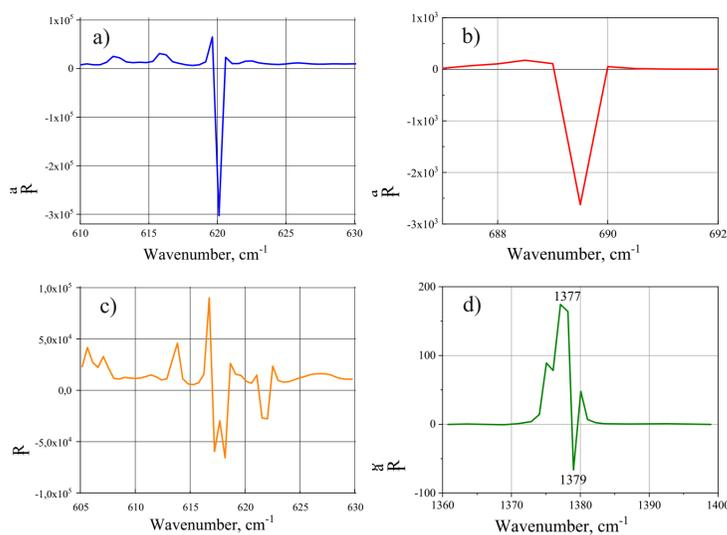
Fig. 5. Two-polar IR absorption in macroporous silicon structures (a, c) and “polymer (PVC)–CNTs” composites (b, d).
