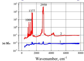
Fig. 4. IR absorption spectra of polypropylene (1) and “polypropylene-CNTs” composite (2).
