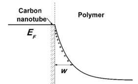
Fig. 3. Band bending and SCR width  $w$  at the “polymer-CNTs” boundary.
