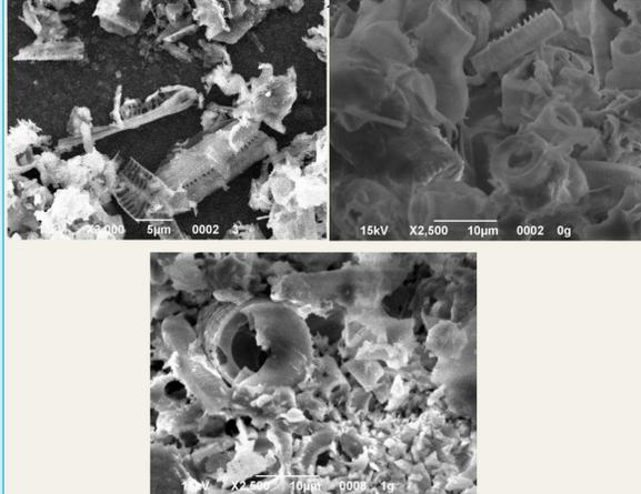
Fig. 1 Photomicrographs of samples a— diatomite, b- diatomite-alginate, c- diatomite-alginate- Fe<sub>3</sub>O<sub>4</sub>
