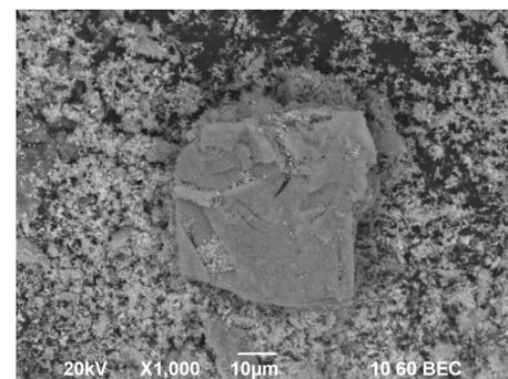
Fig.2. SEM image of initial mixture ZnO and  $V_2O_5$
