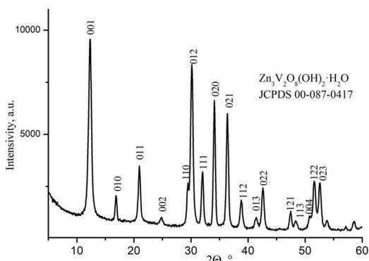
Fig.3. XRD data of ZnO and  $V_2O_5$  after US treatment
