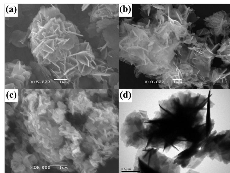
Fig.4., SEM images of ZnO and  $V_2O_5$  after (a) US, (b) BT and (c) MCh treatment, (d) TEM image of  $Zn_3V_2O_7(OH)_2 \cdot 2(H_2O)$
