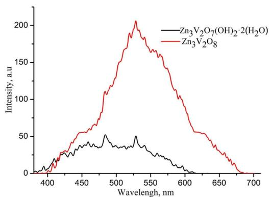
Fig.5 PL spectra of  $Zn_3V_2O_7(OH)_2 \cdot 2(H_2O)$  and  $Zn_3V_2O_8$  ( $\lambda_{ex} = 360$  nm).
