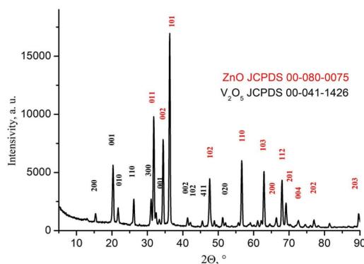
Fig.1. XRD data of initial mixture ZnO and  $V_2O_5$
