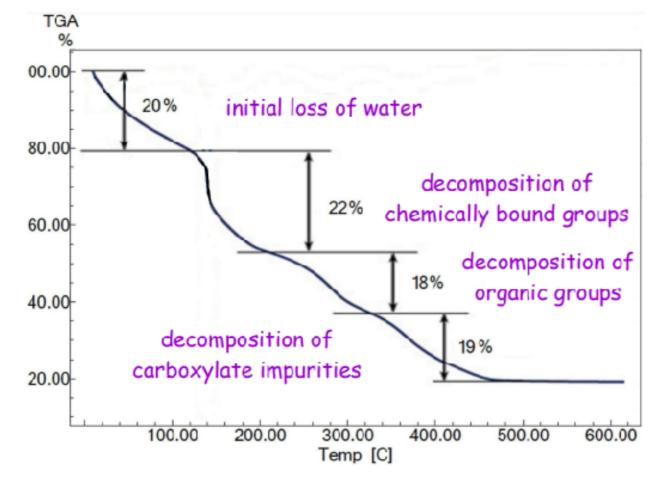
Fig.1. The thermogravimetric curve of the gel.
