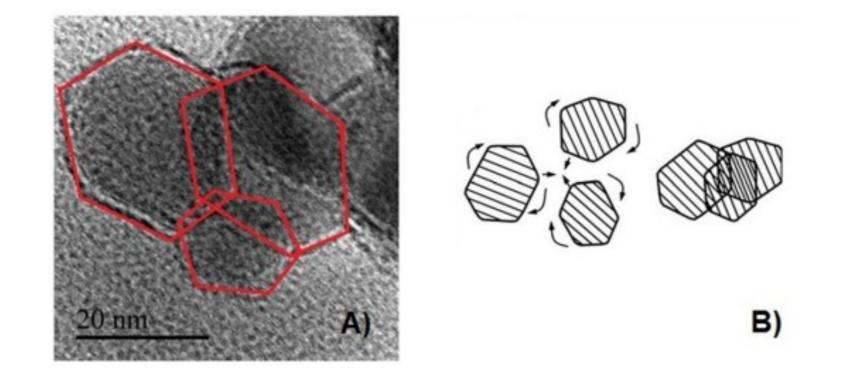
Fig.2. Oriented consolidation (attachment) of ZnO nanoparticles: (A) HRTEM image, calcinations temperature 500 °C, (B) scheme of mechanism.
