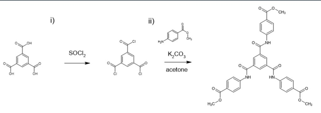
Fig. 1. Synthesis of 4,4',4"-[1,3,5- benzenetriyltris(carbonlimino)]trisbenzoic acid methyl ester.
