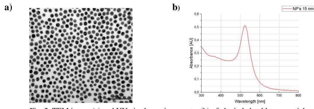
Fig. 2. TEM image (a) and UV-vis absorption spectra (b) of obtainded gold nanoparticles.
