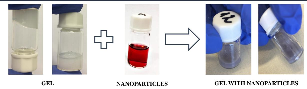
Fig. 3. The proces of obtaining supramolecural gel with gold nanoparticles.
