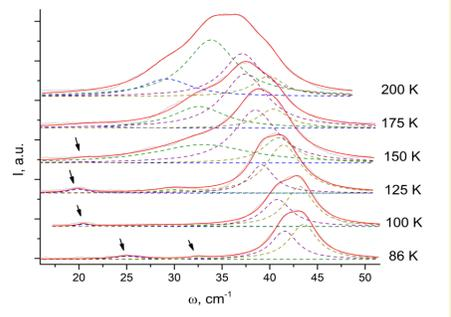
Fig. 5. The low frequency part of Raman scattering spectra for ferroelectric phase of  $\text{CuInP}_2\text{S}_6$  crystal at several temperatures.
