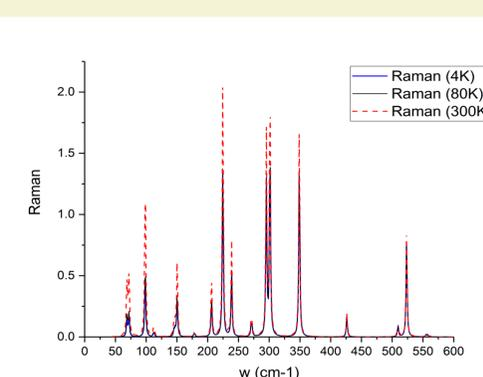
Fig. 4. Calculated in GGA approach Raman scattering spectra for  $\text{CuInP}_2\text{S}_6$  crystal at different temperatures.
