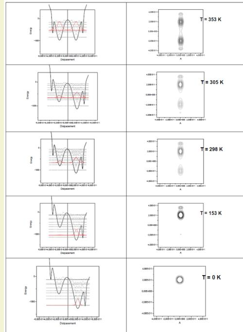
Fig. 7. Shape of the local potential determined following thermal evolution of different copper site occupancies and the corresponding probability density contours in  $\text{CuInP}_2\text{S}_6$  crystal.
