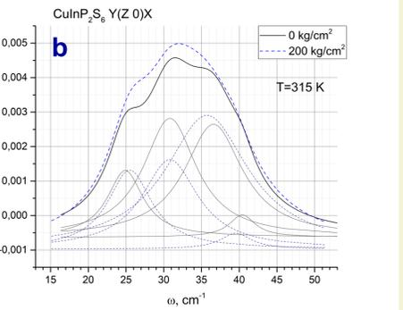
Fig. 6. The low frequency part of Raman scattering spectra for  $\text{CuInP}_2\text{S}_6$  crystal at different temperatures (a) and under uniaxial pressure normally to structural layers (b).
