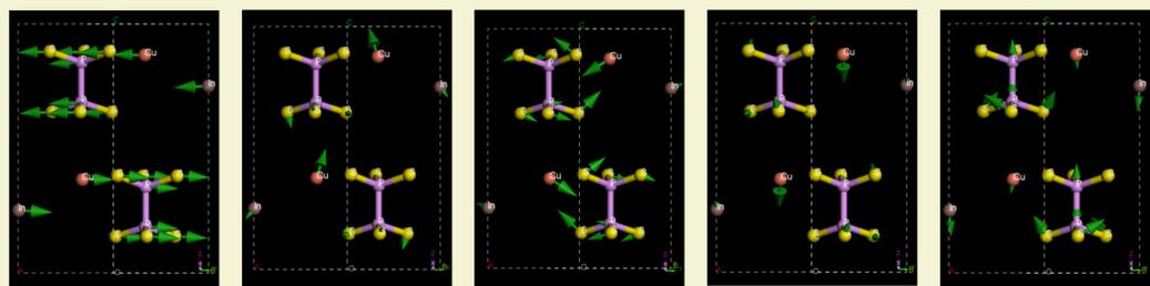
Fig. 3. Eigenvectors of the low frequency optical lattice vibrations at center of Brillouin zone for ferroelectric phase of  $\text{CuInP}_2\text{S}_6$  crystal.
