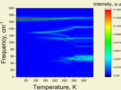
Fig. 9. Calculated in the four – well quantum anharmonic oscillators model temperature dependence of the pseudospin fluctuations spectra intensities.
