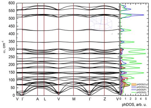
Fig. 2. Calculated in GGA approach phonon branches and partial phonon densities of states for ferroelectric phase of  $\text{CuInP}_2\text{S}_6$  crystal.
