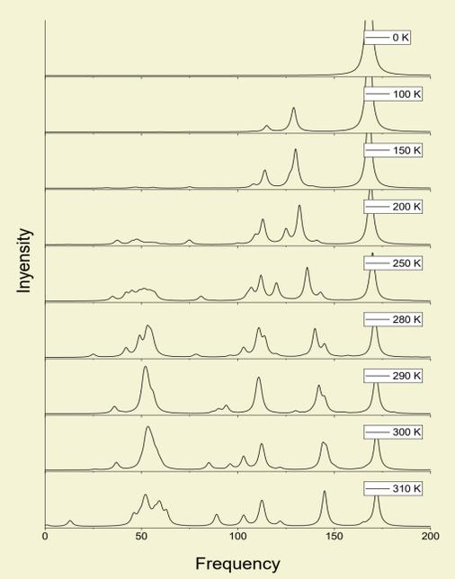
Fig. 8. Calculated in the four – well quantum anharmonic oscillators model temperature transformation of pseudospin fluctuations spectra at shown on Fig. 7 temperature variation of the local potential.
