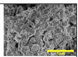
According to XRD, SEM and TEM data, it has been found that 0.8BLFO-0.2MZFO composite is a combination of multiferroic  $Bi_{0.9}La_{0.1}FeO_3$  (BLFO) rhombohedral polar R3c and ferromagnetic  $Mn_{0.6}Zn_{0.3}Fe_{2.1}O_4$  (MZFO) cubic ferrospinel Fd3m fractions, an average particle size of which is 160 and 12 nm for BLFO and MZNO, respectively.
