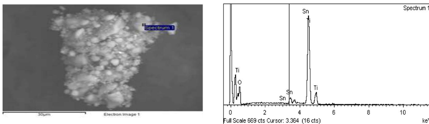
**Fig 1. SEM images and energy-dispersive spectrometry (EDS) spectrum of 2Sn/TiO<sub>2</sub>**
