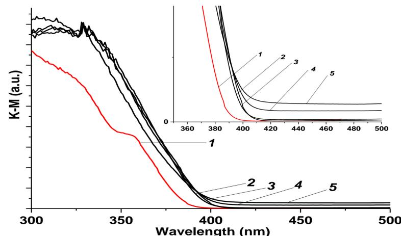
**Fig. 3. UV-Vis diffuse reflectance spectra of samples: 1 – TiO<sub>2</sub>, 2 – 0.1Sn/TiO<sub>2</sub>, 3 – 0.5Sn/TiO<sub>2</sub>, 4 - 1Sn/TiO<sub>2</sub>, 5 - 2Sn/TiO<sub>2</sub>**
