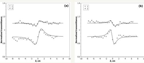
**Fig.3.** Closed aperture Z-scan results at  $\lambda = 1064$  nm: (a) is for the sample at T<sub>S</sub> = 293K, 1.0Pa (1) and 3.0Pa (2); (b) is for the sample at T<sub>S</sub> = 293K, 5.0Pa (1) and T<sub>S</sub> = 800K, 1.0 Pa (2). Marks represent experimental data and solid lines are numerical fits to the data using the theory.
