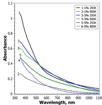
**Fig.2.** The linear optical absorption properties of nano-scale copper oxide films deposited, by RPLD on SiO<sub>2</sub> substrates: at P(O<sub>2</sub>) = 1.0Pa, T<sub>S</sub> = 293K (1) and T<sub>S</sub> = 800K (2); P(O<sub>2</sub>) = 3.0Pa, T<sub>S</sub> = 293K (3) and T<sub>S</sub> = 800K (4); P(O<sub>2</sub>) = 5.0Pa, T<sub>S</sub> = 293K (5) and T<sub>S</sub> = 800K (6)
