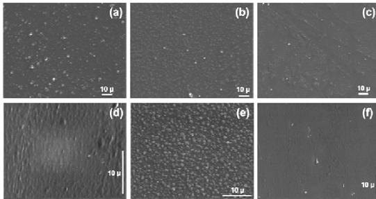
**Fig.1.** SEM images of nano-scale copper oxide films deposited by RPLD on SiO<sub>2</sub> substrates: at P(O<sub>2</sub>) = 1.0Pa, T<sub>S</sub> = 293K (a), P(O<sub>2</sub>) = 3.0Pa, T<sub>S</sub> = 293K (b), P(O<sub>2</sub>) = 5.0Pa, T<sub>S</sub> = 293K (c) and P(O<sub>2</sub>) = 1.0Pa, T<sub>S</sub> = 800K (d), P(O<sub>2</sub>) = 3.0Pa, T<sub>S</sub> = 800K (e), P(O<sub>2</sub>) = 5.0Pa, T<sub>S</sub> = 800K (f)
