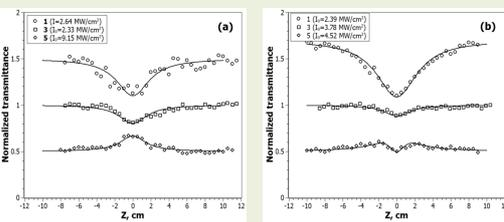
**Fig.6.** Open aperture Z-scan results at  $\lambda = 532$  nm (a) is for the sample at T<sub>S</sub> = 293K and 1.0Pa (1), 3.0 Pa (2), 5.0 Pa (3) (b) is for the sample at T<sub>S</sub> = 800K and 1.0Pa (1), 3.0Pa (2), 5.0Pa (3). Marks represent experimental data and solid lines are numerical fits to the data using the theory.
