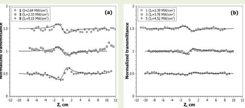
**Fig.5.** Closed aperture z-scan results at  $\lambda = 532$  nm for the sample at T<sub>S</sub> = 293K, 3.0Pa. Marks represent experimental data and solid lines are numerical fits to the data using the theory.
