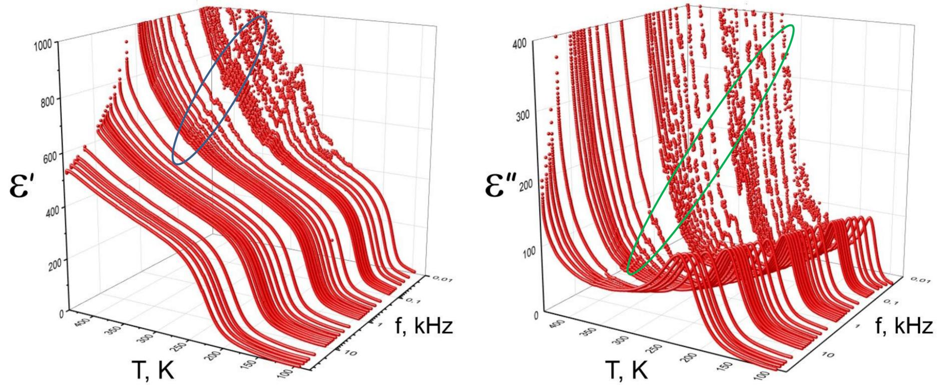
Fig. 1. Temperature dependence of real and imaginary part of dielectric permittivity of Cu<sub>0.15</sub>Fe<sub>1.7</sub>PS<sub>3</sub>. The highlighted area indicates anomalies at 373K.
