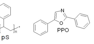
Chemical structure of the components of pS-PPO NP polystyrene (PS) and diphenyloxazole (PPO)
