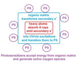
We propose using nonscintillating heavy elements to enhance the quantity of secondary electrons
