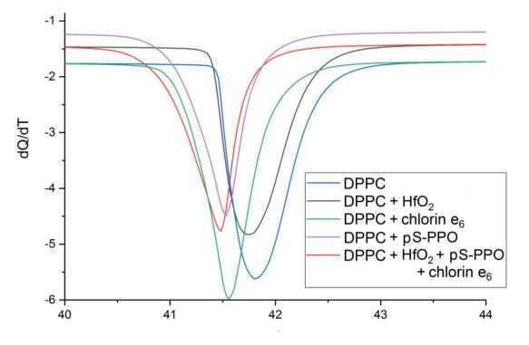
Phase transitions in model membranes of 1,2-Dipalmitoylsn-Glycero-3-Phosphatidylcholine (DPPC) in the presence of  $HfO_2 / pS-PPO / chlorin e_6$  nanosystem and its components.
