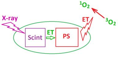
Scheme of traditional approach to construct X-ray PDT sensitizer. Scint scintillating NP; **PS** – photosensitizer; **ET** – excitation energy transfer.
