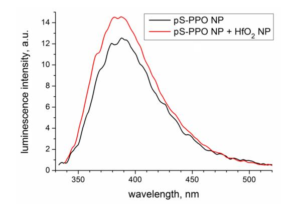
X-ray luminescence spectra of pS-PPO NP and mixture of pS-PPO NP (black) and HfO<sub>2</sub> NP (red).
