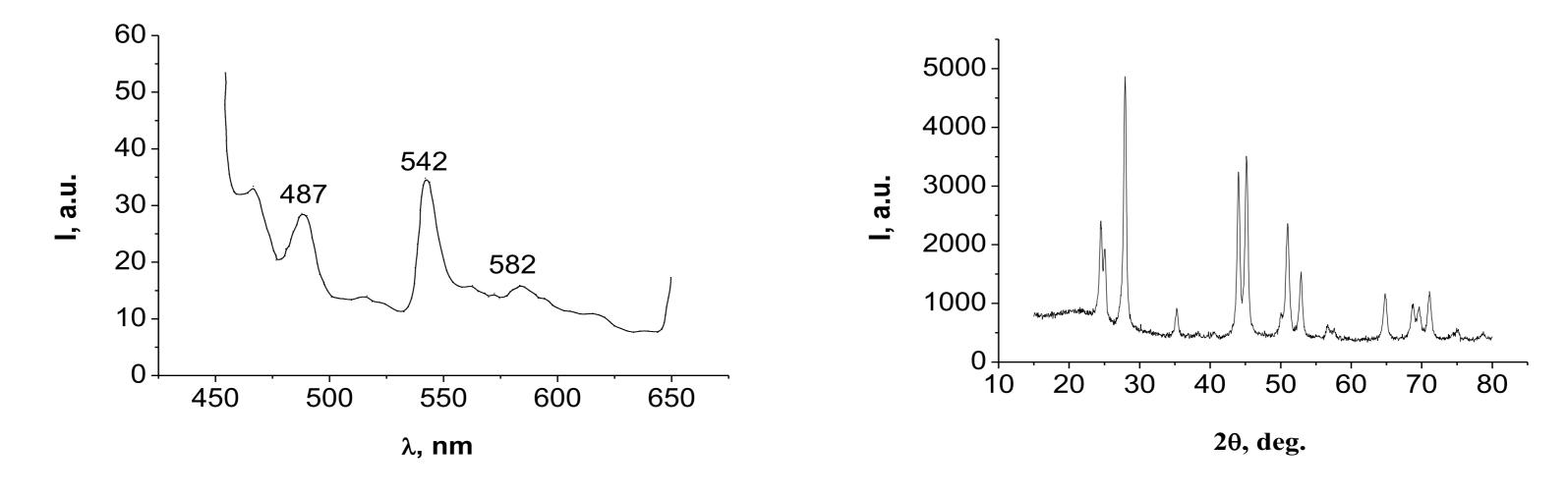
Luminescent spectrum of aqueous dispersion containing NPs LaF<sub>3</sub>:Tb under 254 nm UV excitation
