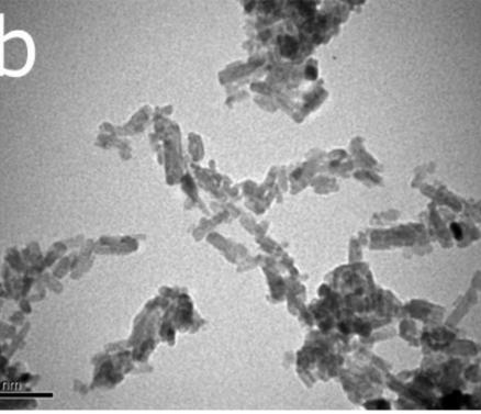
TEM images of nanoparticles LaF<sub>3</sub>:Tb. Scale bar 20 nm (a); 50 nm (b)
