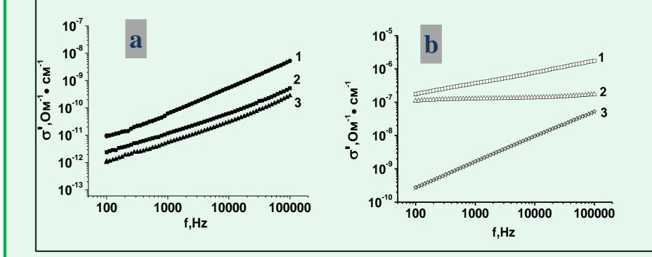
Dependences of the conductivity vs frequency for SPE membranes based on TBC1 (**a**) and TBC<sub>hydr</sub> (**b**): without dopant  $-3(\mathbf{a})$ ,  $3(\mathbf{b})$ ; dopted with LiPF<sub>6</sub> at molar ratio [PEO]/[LiPF<sub>6</sub>]=0.15  $-2(\mathbf{a})$  and  $2(\mathbf{b})$ ; dopted with LiPF<sub>6</sub> at molar ratio [PEO]/[LiPF<sub>6</sub>]= 0.06  $-3(\mathbf{a})$ and  $3(\mathbf{b})$ . T=25 °C.
