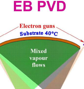
Physical synthesis silver of nanoparticles (NPs) by the method of condensation of mixed molecular flows in vacuum (EB PVD) allows obtaining nanostructured material (16 wt. % Ag-NaCl) in the form of a dry substance (silver NPs in a watermatrix), which soluble allows preserving, storing and transporting the nanoparticles.
