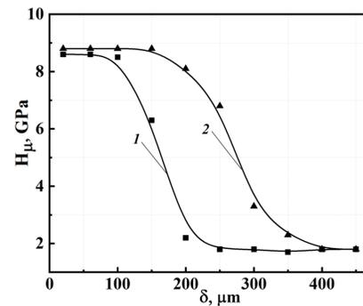
Fig. 2. Microhardness of the surface layer of 40Kh steel after MPT by different tools: 1 - with plane surface; 2 - with multidirectional inclined grooves.
