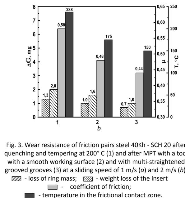
Fig. 3. Wear resistance of friction pairs steel 40Kh - SCH 20 after quenching and tempering at 200 °C (1) and after MPT with a tool with a smooth working surface (2) and with multi-straightened grooved grooves (3) at a sliding speed of 1 m/s (a) and 2 m/s (b): ▨ - loss of ring mass; ▩ - weight loss of the insert; ▭ - coefficient of friction; ■ - temperature in the frictional contact zone.
