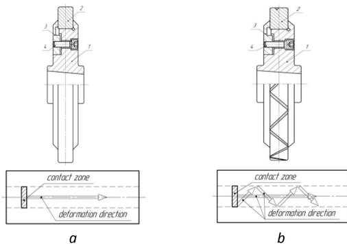
Fig. 1. General view of the used tools: a - with plane surface; b - with multidirectional inclined grooves: 1 - case; 2 - work disk; 3 - flange; 4 - screw.
