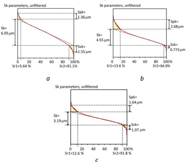
Fig. 4. Support curves of friction pairs steel 40Kh - SCH 20 after quenching and tempering at 200 °C (a) and after MPT with a tool with a smooth working surface (b) and with multi-straightened grooved grooves (c)
