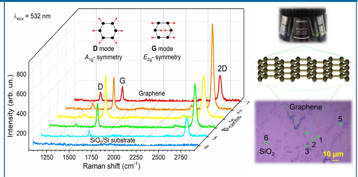
Raman spectra of a graphene monolayer on a  $Si/SiO_2$  substrate at different points on the surface and an image of this layer in the objective lens of an optical microscope.
