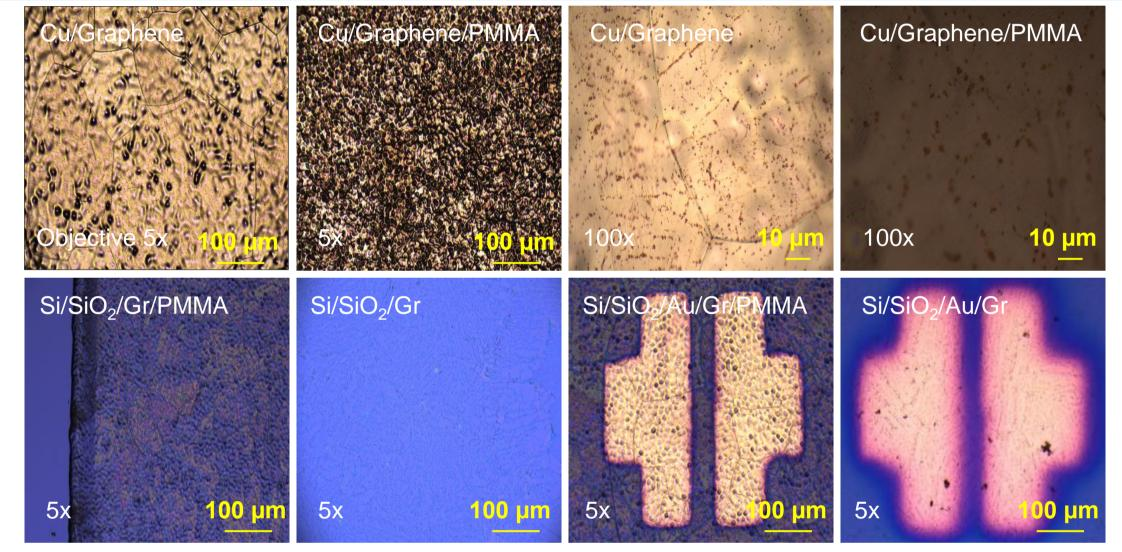
Optical surface morphology of graphene layer on Cu foil and covered by PMMA. Graphene layer transferred to  $Si/SiO_2$  substrate with prepared Au contacts.
