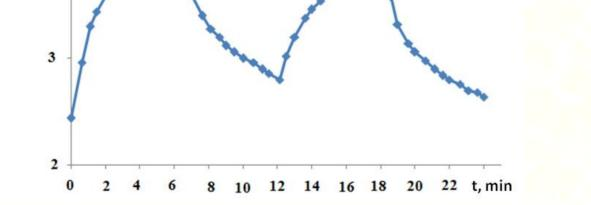
*Fig. 6. Relaxation of current in ZnO film at periodic* inflow into the chamber of water vapor or dry air (V = 200 B) at T = 293 K.
