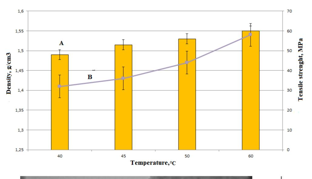
Dependences of density (A) and tensile strength (B) of nanocellulose films on temperature and acid concentration
